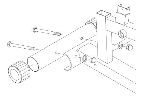
Attach front foot tube (27) to frame (1) using: Qty 2 - (37) Carriage Bolt Qty 2 - (39) Flat Washer Qty 2 - (54) Cap Nut
